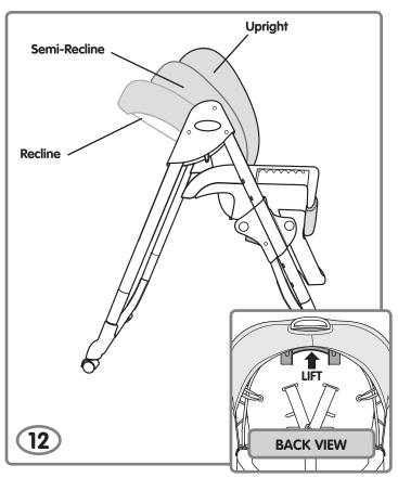
**Hint:** Adjust the seat angle to any of three positions: Upright, Semi-Recline or Recline.
